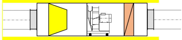
(11) *'thermal efficiency of a non-residential HRS (\eta\_{t\\_nrvu})* means the ratio between supply air temperature gain and the exhaust air temperature loss, both relative to the outdoor temperature, measured under dry reference conditions, with balanced mass flow, an indoor-outdoor air temperature difference of 20 K, excluding thermal heat gain from fan motors and from internal leakages;
