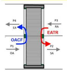
Run-around HRS are connected through a heat transfer system and are not allowed to have any internal leakage, if there is a common wall between the supply and extract air side, then the leakage shall be tested with a differential pressure of 250 Pa in accordance with EN 308 and the leakage have to be negligible (less than 0.1 %). Recuperators can be tested with 250 Pa pressure difference in accordance with EN 308 or with an EATR test. EATR shall be tested for regenerators. EATR is defined as:
